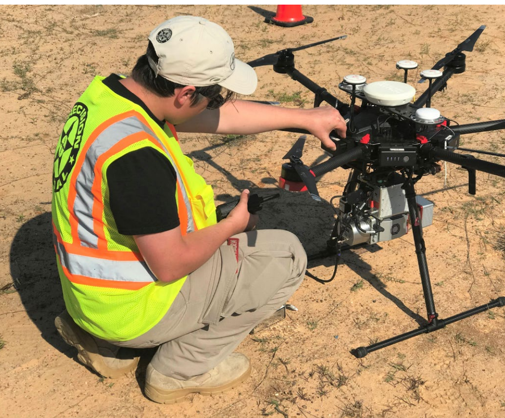
Figure 6: A Precision team member prepares their miniRANGER for the mission. Most lidar systems by Phoenix are modular and can be unclipped from their UAVs and mounted onto vehicles, backpacks, and more.
