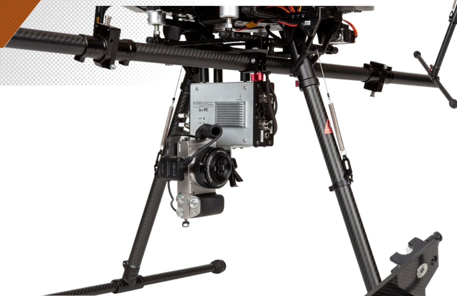
Figure 4: GeoPhotomap. In this view, the Sony camera, mounted below the Navigator system, is pointing horizontally for tower inspection, but the user can rotate it to the vertical for nadir scanning in seconds.
