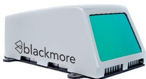
Figure 6: Blackmore's Autonomous Fleet Doppler Lidar (above) and Lidar Development Platform (right) support customers in broader autonomy space with real-time, FMCW lidar. See blackmoreinc.com for more details.
