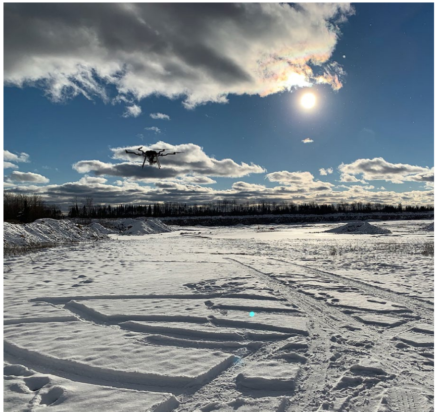
Figure 4: Harris H6 and lidar payload in flight on a frigid day.
