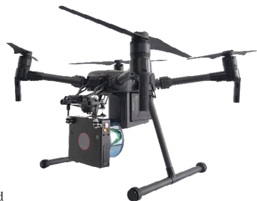
Figure 6: Genius UAV lidar installed on DJI 210.
