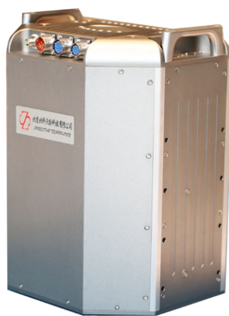
Figure 4: A-Pilot airborne scanner.
