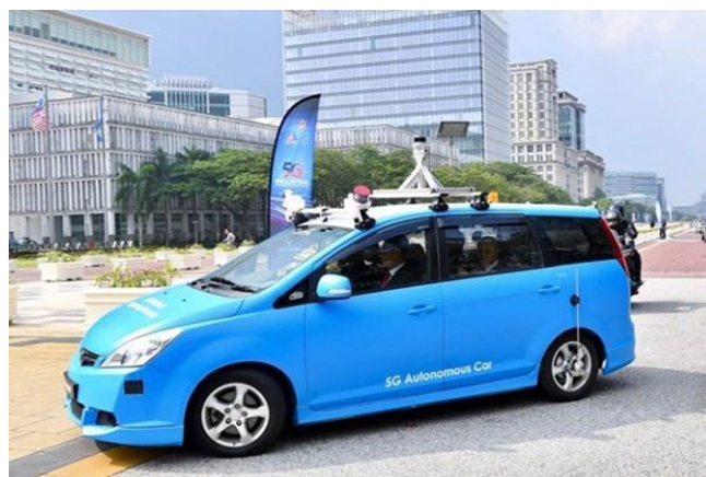
Figure 9: 5G autonomous car of Malaysia equipped with SureStar lidar.
