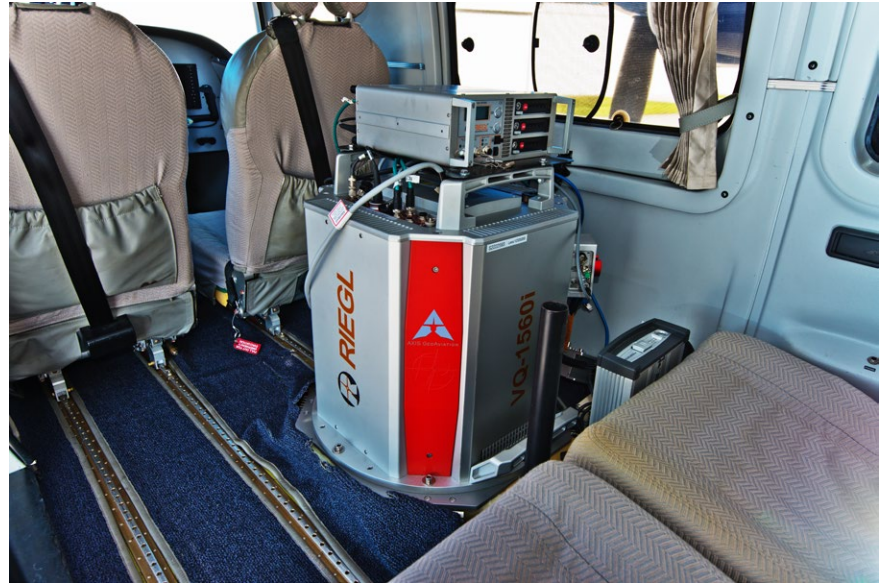
Figure 3: RIEGL LMS-Q1560 lidar sensor mounted in the company's Piper Navajo aircraft (left) and RIEGL LMS-Q1560 lidar sensor mounted in Vulcan Air p68C (middle) and Vexcel UltraCam Eagle F100 (right).
