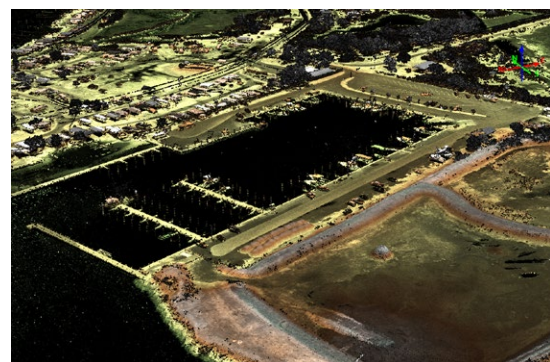
Figure 6: Colorized point cloud of an airport terminal (left) was collected for a FAA 18C obstruction analysis. This view is a combination of the lidar data plus the imagery collected on the same flight. The lidar elevation view of the same airport terminal is shown on the right.
