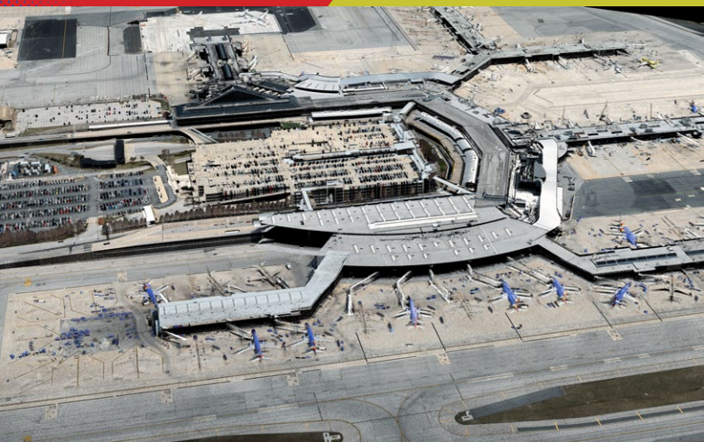
Figure 6: Colorized point cloud of an airport terminal (left) was collected for a FAA 18C obstruction analysis. This view is a combination of the lidar data plus the imagery collected on the same flight. The lidar elevation view of the same airport terminal is shown on the right.
