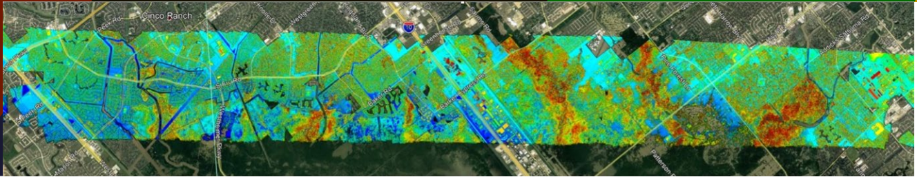
The Windmill Bluff Lane point-cloud is a small subset of this point-cloud covering 50 square miles that was generated from a single scan. Analysts applied the same algorithms that automatically identified debris in that neighborhood to the entire dataset; debris is highlighted below.
