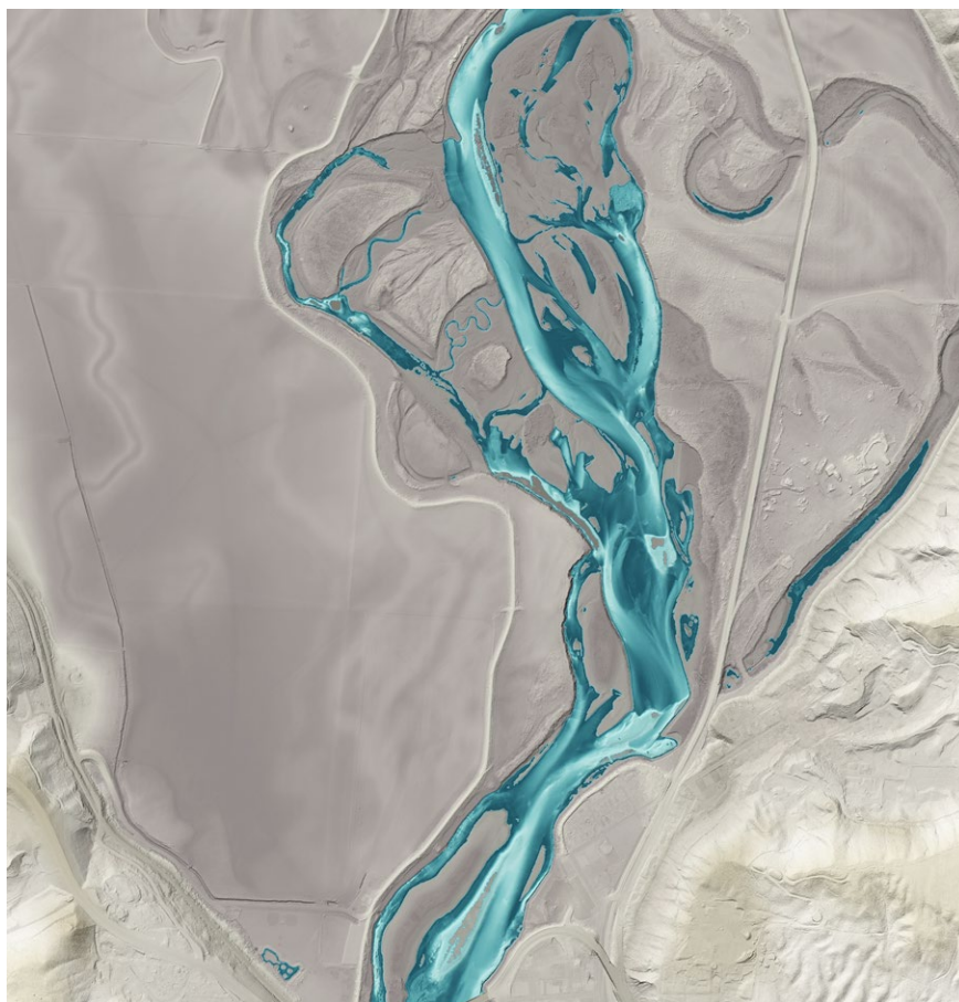
An integrated lidar-derived topobathymetric model showing the extensive river braiding, depicting both bare earth (grey) and subsurface bottom (blue) terrain.
