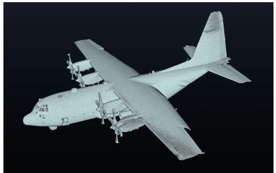
Figure 5: C-130 Hercules point cloud captured and processed with Kaarta Stencil
