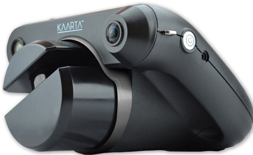
Figure 3: Kaarta Contour integrated mobile mapping system.
