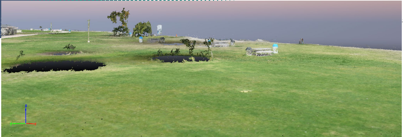
Figure 2: UAV photogrammetry: examples where photogrammetry fails: scale mismatch and missing data under foliage, trees and canopy.
