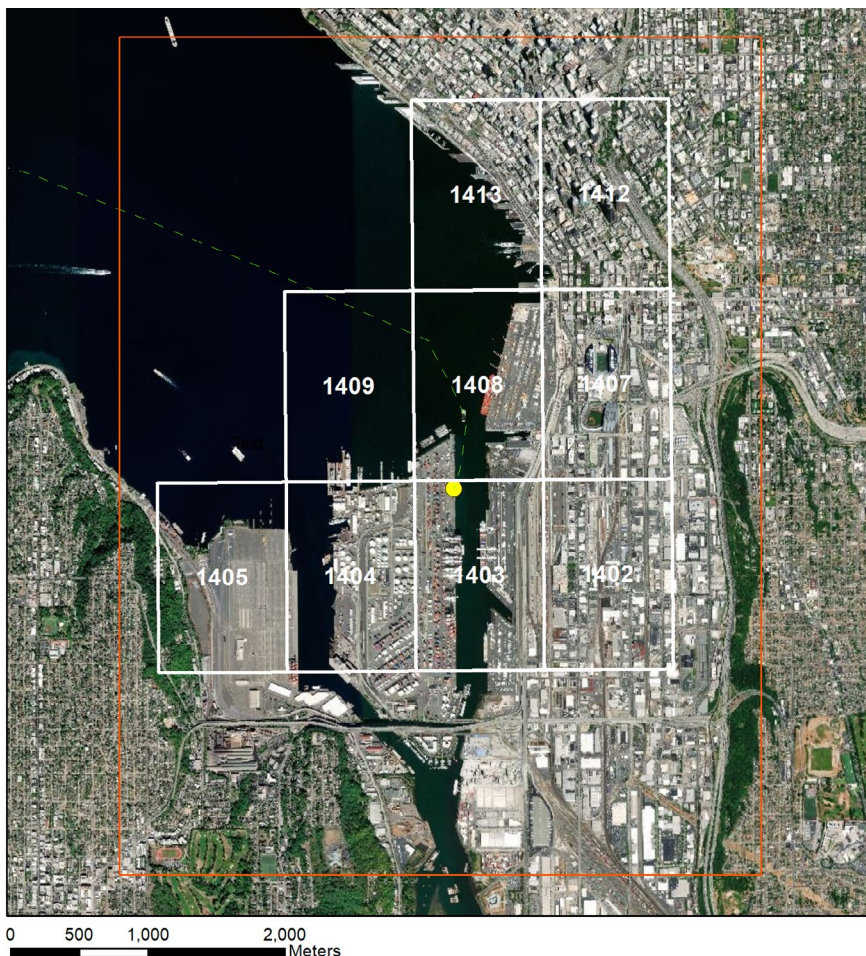
Figure 2: The extent of the lidar processing is defined by the nine tiles displayed within the Area of Responsibility (red outline). LAS files were merged using LAsTools, and projected to UTM 10N WGS 84 then classified into ground, buildings and vegetation. The classified LAS file was imported into a Terrain Product, along with an extent boundary, and a simplified water polygon representing Elliot Bay for hydroflattening. Base data source: Esri, DigitalGlobe, GeoEye, Earthstar Geographics, CNES/Airbus DS, USDA, USGS, AeroGRID, IGN, and the GIS User Community.
