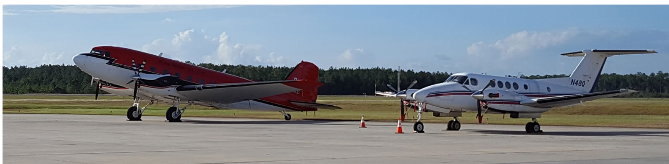
The Dynamic Aviation King Air 200 (right) and Kenn Borek Air Basler BT-67 were used in the post-Matthew lidar collection, carrying the CZMIL sensor, owned by USACE and JALBTCX.
