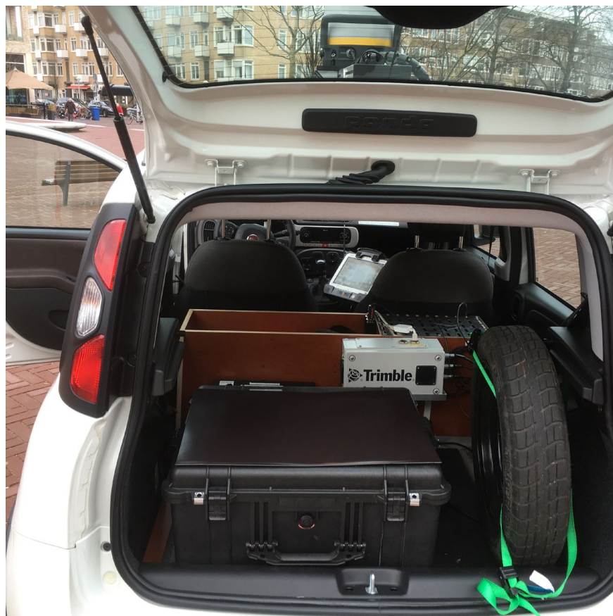
The MX7 system installed in a vehicle. The hardware is readily transferred to other vehicles or boats.
