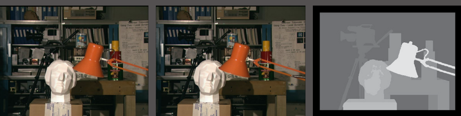
Figure 1: Left and right images of a stereo pair and the “disparity” map (right) showing the differences of each pixel in the right and left image.
