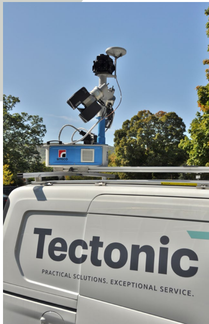
Figure 2: close up view of the SITECO Roadscanner Compact with Faro scanners
