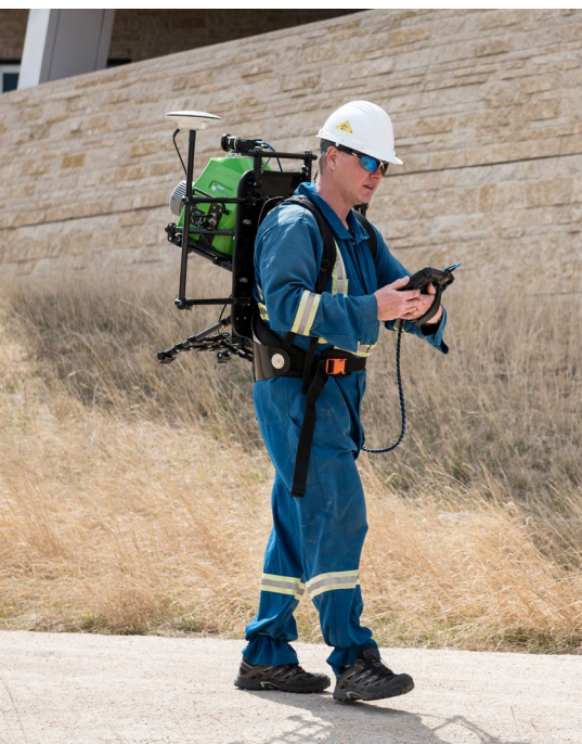
The ROBIN Mobile mapping system being used in backpack set-up.
