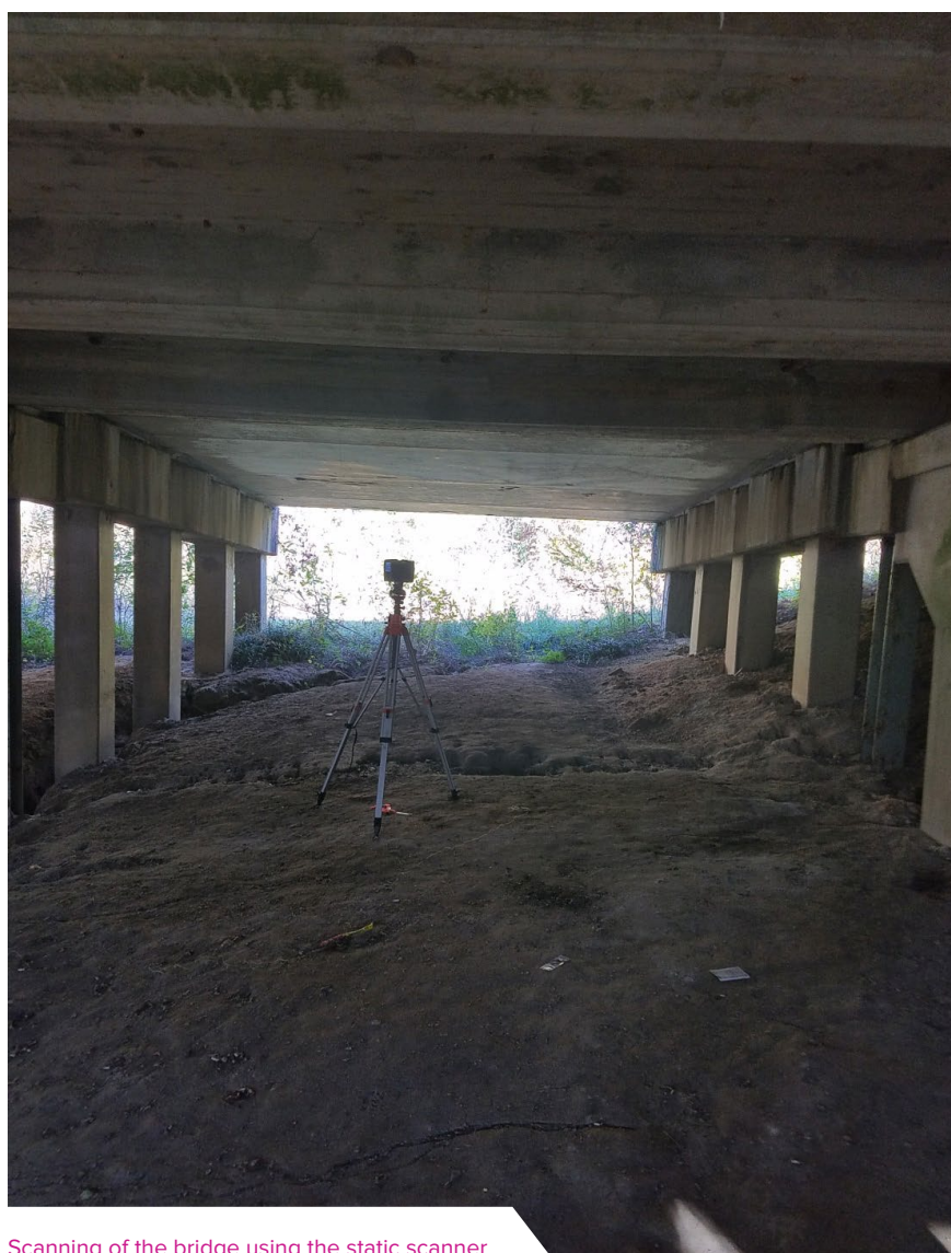
Scanning of the bridge using the static scanner
