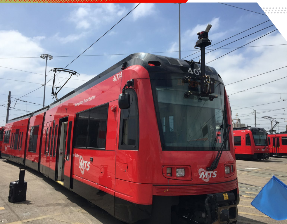
Maverick mounted to a commuter train with Mandli's prototype suction cup mount. The mount is powered by a vacuum pump with an internal backup battery housed within the control box.
