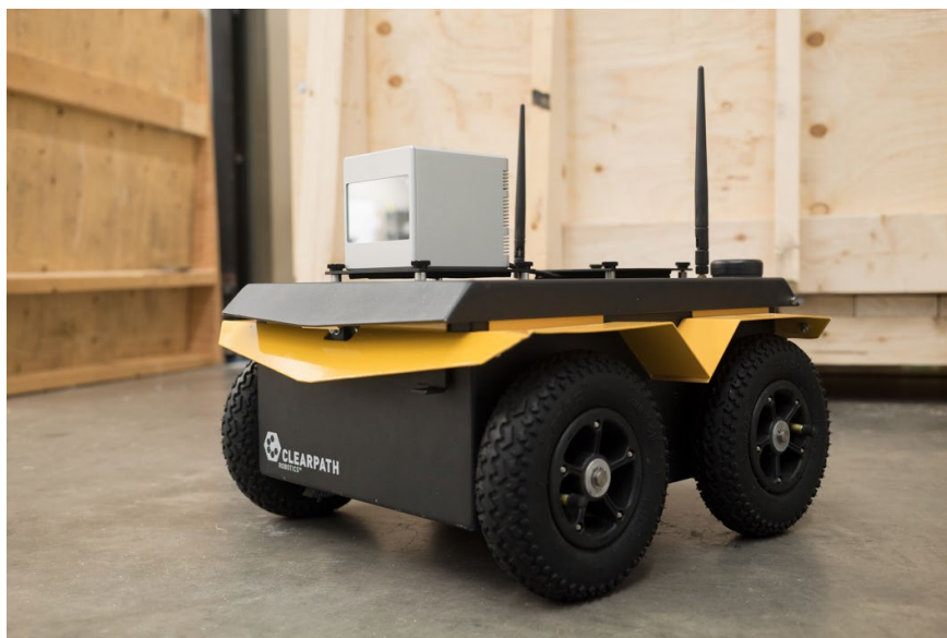
Figure 7: Cepton HR80W mounted on Clearpath Husky warehouse robot.
