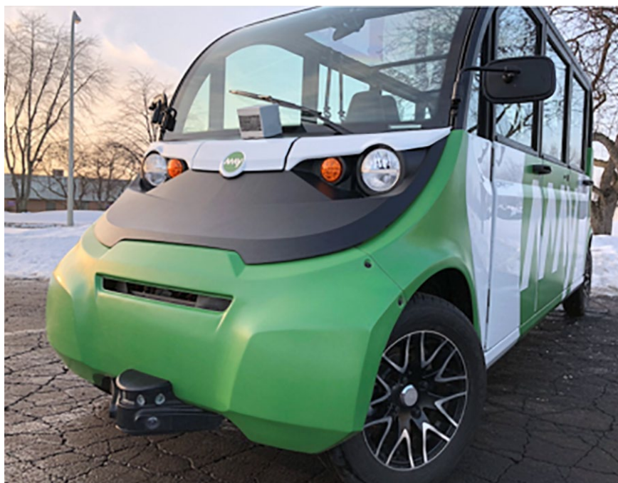
Figure 8: Cepton HR80W mounted on May Mobility autonomous vehicle.
