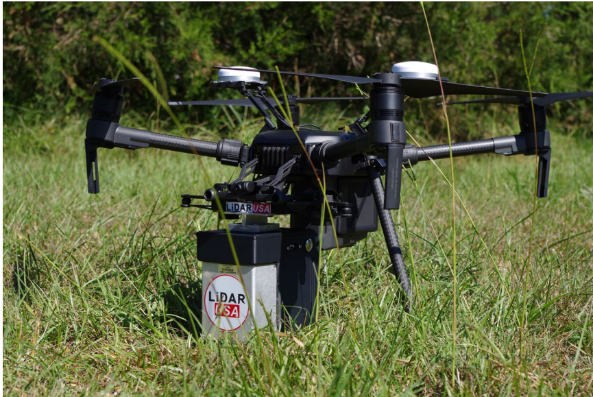
Figure 5: Cepton SORA 200 integrated on to UAV lidar system by LiDAR USA.
