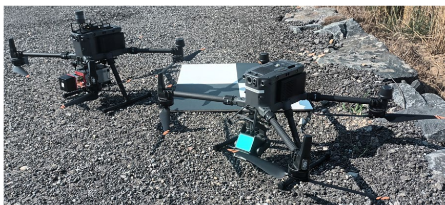
Figure 5: Integration example: RIEGL miniVUX-3UAV (left) and DJI Zenmuse L2 (right), each mounted on a DJI Matrice 350 RTK multicopter UAV.
