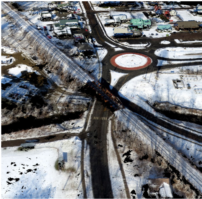
Figure 4a: UAS photogrammetric point cloud (same location as 4b).
