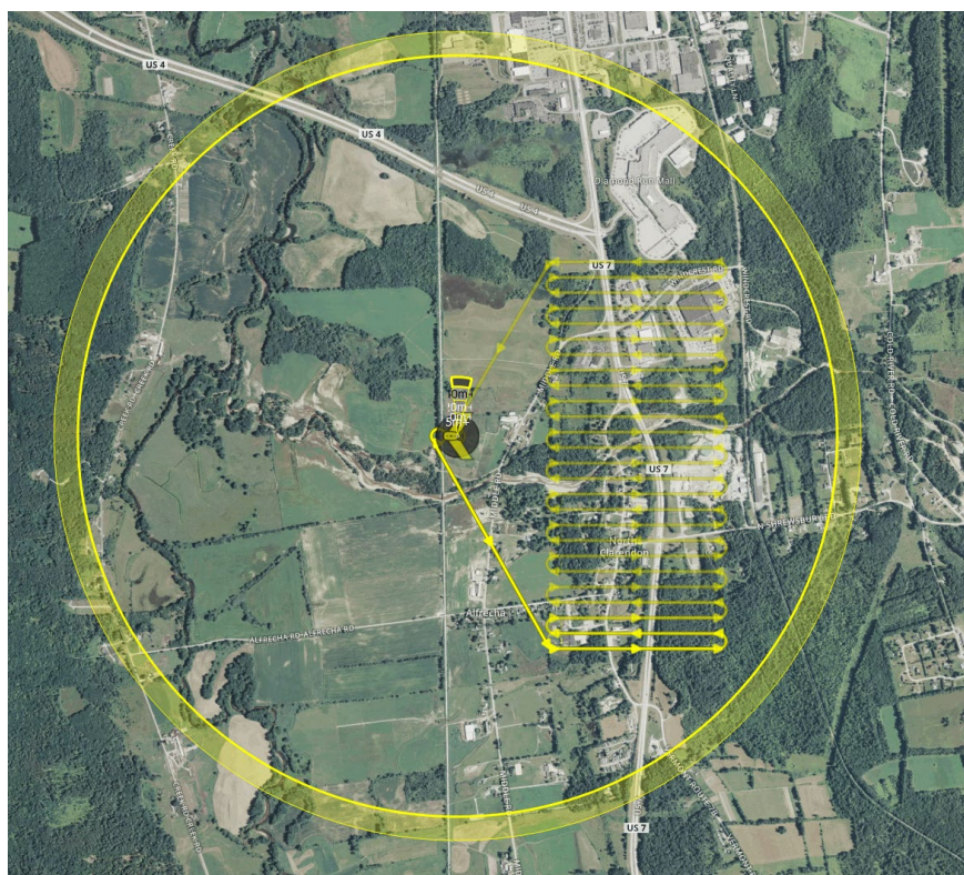
Figure 1: Sample UAS flight plan generated with eMotion software suitable for producing a photogrammetric point cloud.
